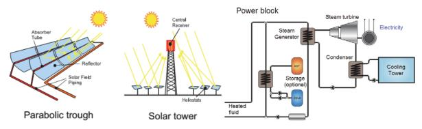
Fig.7 Parabolic and solar tower systems, and the power block used for electricity generation
