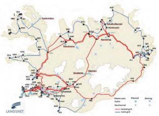
Fig. 10 Plans for network development until 2025.
