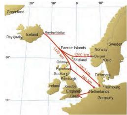
Fig. 13 Possible HVDC connections to the mainland of Europe.
