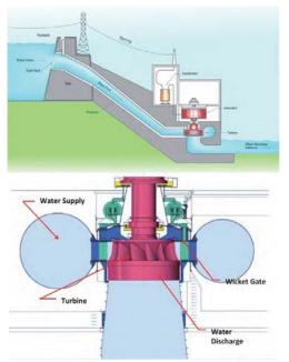
Fig. 5 Above: The common principle used in Icelandic hydro plants. Below: The Francis turbine.
