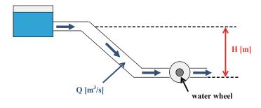
Fig.1 Principle of hydroelectric power generation.
