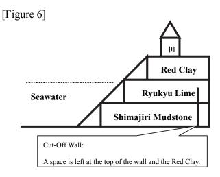
The water content of the red clay is only about 10%. Most rainwater is not retained in the soil; it flows into the sea. Therefore, it is really important for the island to have this kind of dam.
