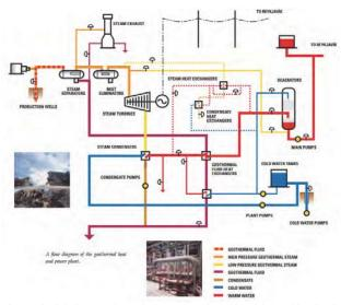
Fig. 8 Principle in a geothermal plant, where both electricity and heating is produced.
