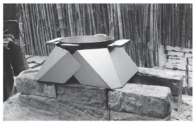
Figure.6 A final prototype of pot skirt attached to a traditional biomass cookstove
