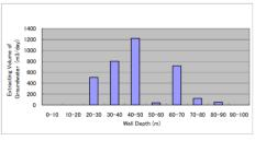
Fig. 3. Well depth and extracted volume of groundwater by several depth of private wells [4].
