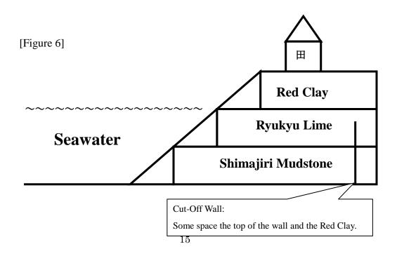
The water content of the red clay is only about 10%. The most of water from rain is not saved into the soil. It almost flows into the sea. Therefore, it is really important for the island to have the kinds of dam. The suitable conditions for the subsurface dams are that first, the soil is easy to carry water, second, the land has lots of rain and finally the topography of the underground is like valleys. Thus, Miyakojima Island is suitable for subsurface dams.
